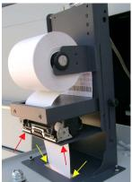
Close the roller door (red arrows) and feed the extra paper through the slot on the printer door (yellow arrows).
