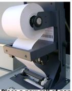
Place a new roll of paper on the spindle with the thermal side facing out (while feeding the paper, the thermal side will be facing back toward the printer body). Feed the paper as shown above.
