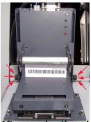
After opening the printer door, loosen the two thumb screws (red arrows) on either side of the printer.
