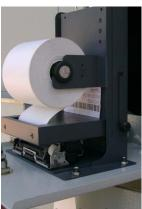
Loosen the thumb screws, lower printer body to the lower rest notches and tighten the thumb screws.
